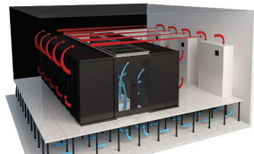
Cooling & Heat Containment Systems
