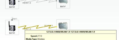
Reason: Warning: BAT-F/WLAN Interface 1/WLAN 1.9/Signal to Noise Ratio<16, Current Value:13
